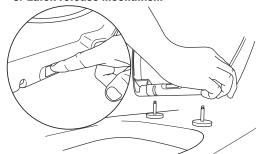
This toilet seat is designed for quick and easy removal when cleaning the toilet pan. To activate the quick release lift up the lid and seat ring, then press the button in the centre of the hinges and lift. To replace the seat align the sockets with the pins and firmly press into position.
