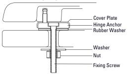
Maximum adjustment of the pin position is achieved by rotating the hinge anchor around the screw (adjustment A in the parts diagram above). Further fine adjustment of the pin position can be achieved by sliding the screw in the adjustment plate (adjustment B).
