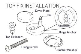
Maximum adjustment of the pin position is achieved by rotating the hinge anchor around the screw (adjustment A in the parts diagram above). Further fine adjustment of the pin position can be achieved by sliding the screw in the adjustment plate (adjustment B).
