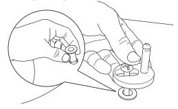
Place the Top Fix Inserts into the fixing holes in the toilet pan. Insert the screws within the Hinge Anchors as shown and begin to tighten the screws until they are loosely secured, to allow for adjustment of the seat on the pan.
