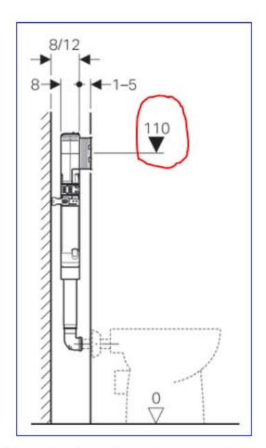
Measurement is taken from the centre of the flush plate the finished floor level (110mm)
