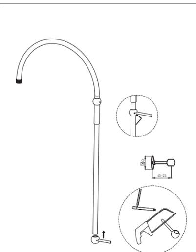
**2** Cut the pole to the required length to align with the shower valve. Screw the pole into the wall bracket. Install the wall bracket onto the long pipe. Lock the grub screw with an Allen key.
