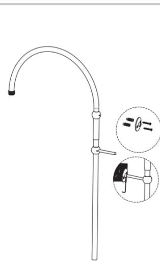
**3** Drill two holes with required height. Fix the back plate onto the wall with the plugs and screws. Insert the pole into the back plate and lock the grub screw with an Allen key.
