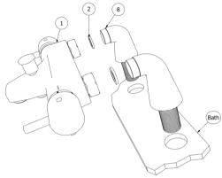
With the pillars loosely attached the pillars can be inserted through the holes on to the bath.
