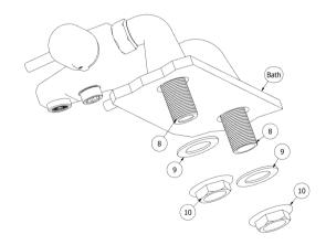
Once the pillars are inserted the back nut washer (9) can be placed over the thread followed by the back nut (10). With the whole setup loosely tightened perfect alignment can be gained. Once aligned tighten the body onto the pillars along with the back nuts. Once the product is installed onto the bath the water outlets may be attached to the ends of the pillars using the appropriate spanner.
