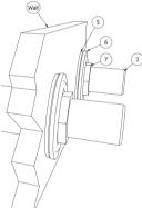
Looking at the wall from front on the wall shrouds (4) may be screwed over the protruding unions (3) and fixed tight up to the wall.
