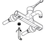
8 - Refit the hot inlet plug into the hot position and the cold into the cold position and refit the covers
