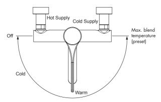
As the handle is rotated anti-clockwise from the off position the delivered water progresses from cold, through warm to the pre-set maximum temperature of approximately 43°C.
