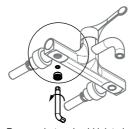
4 - Remove hot and cold inlet plugs using a 10mm Allen key
