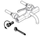
9 - Unscrew the connector plug using suitably sized spanner and refit the check valve assembly and end cover
