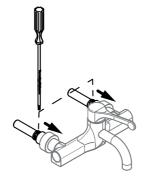
2 - Ensure both isolation valves are in the closed position
