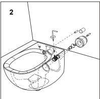
2. Fit wall fixings into the WC as shown. Ensure the flat section on the fixing stud point upward.
