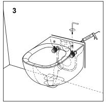
3. Locate the WC on the fixing studs and using the key provided securely tighten each wall fitting.
