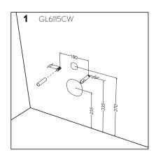
1. Install installation frame in accordance with manufacturers instructions. Set out as detailed to the left
