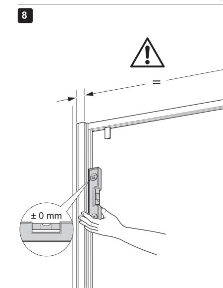
(a) Centralise the door frame within the wall channels, making sure that the door frame is square.
