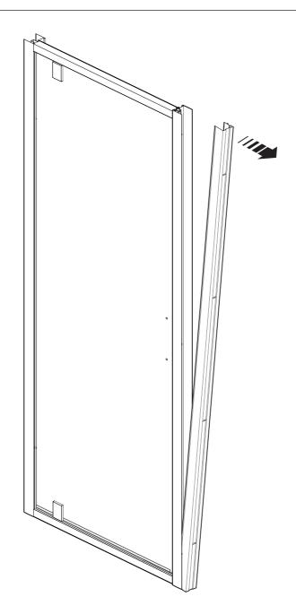
(a) Remove the wall channel.from the door.
