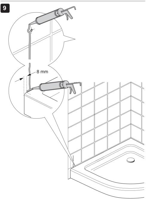
(a) Apply silicone sealant along the length of the wall and at the bottom where the wall channel will be placed.
