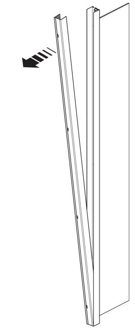
(a) Remove the wall channel.
