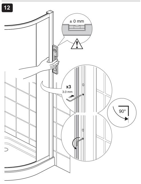
(a) Using the 3.0 mm hexagonal wrench (supplied), turn through 90° clockwise to lock the door frame in position.
