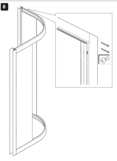
(a) Install the screws to both sides to secure the assembly.
