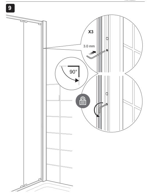
(a) Using the 3.0 mm hexagonal wrench (supplied), turn through  $90^{\circ}$  clockwise in three locations to lock the door frame in position.
