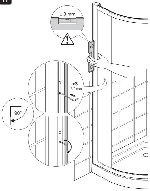
(a) Using the 3.0 mm hexagonal wrench (supplied), turn through  $90^{\circ}$  clockwise to lock the door frame in position.
