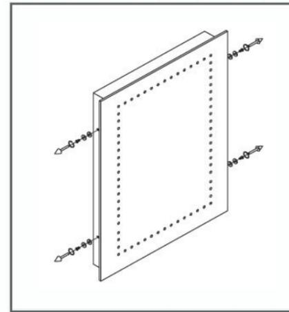
Lay the mirror on a flat surface with the front glass facing upwards. Using a Philips screwdriver, remove the four screws, along with the metal and white spacers on the sides of the mirror as shown above. Carefully lift the mirror off the back box and position it onto a soft flat surface to avoid scratching the mirror. Pierce the small protective IP rated rubber grommet (this will isolate and trap any steam to ensure maximum safety during use).
