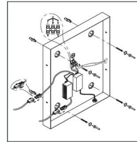
Insert a 3-core cable through the pierced hole in the protective cover, then thread the cable through from behind the back box into the power supply. Mark the position of the fixing holes in the metal back box onto the wall, carefully avoiding any wiring or water pipes. Next, drill and prepare the holes for the screws ensuring that the wall is a solid material. Mount the metal back box of the mirror onto the wall and secure tightly.
