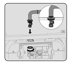
Attach the isolation valve to the cold water supply.
