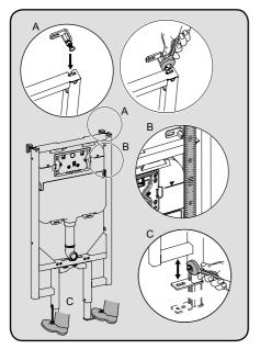
Attach the wall bracket as shown. Set the frame height so the indicated line is 1000mm above the floor level. Tighten the bolts on the frame legs until secure.
