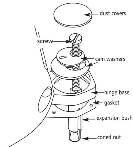
1. Place the seat onto the WC with the pillar hinge bases and gaskets over the seat fixing holes.
