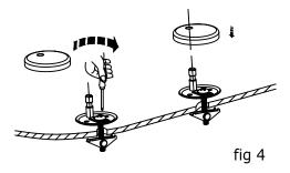
5. Using a crosshead screwdriver completely tighten the pan seat fixings taking care not to move their position. Fit the pan and seat fitting covers (B).
