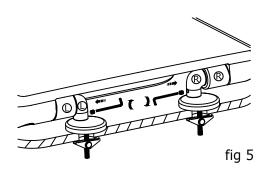
6. Place seat and lid back on to the location pins on the pan fixings and then use hex key provided to tighten grub screws found on the soft close barrels as per figure-5.
