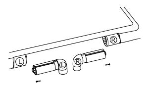
3. Insert the soft close barrel into the houseing hole on each side of left and right.
