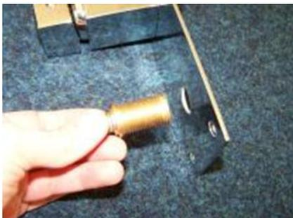
Push the threaded part through the plate from the front.
