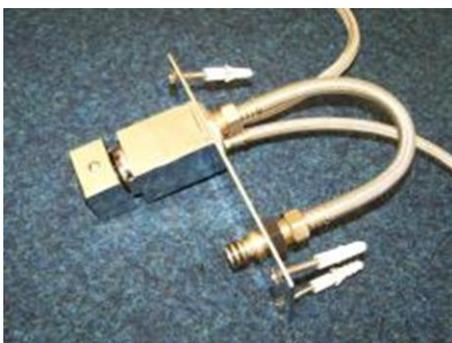
Using the mirror screws and wall plugs provided, fix the assembled plate into the wall, after the plumbing connections have been made. The joints should be checked for leaks. Note: A wall baton may be needed to attach the screws into to make a solid fix. A small bead of silicone sealant needs to be added to the back of the plate to make a water tight seal.
