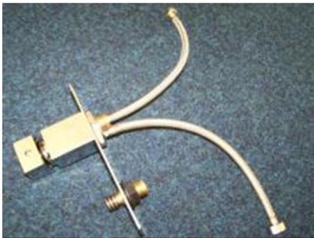
Attach in the flexible inlet pipes. Do not over tighten. These are to be plumbed into hot & cold water supplies. Flush out the pipes prior to this to remove any debris.
