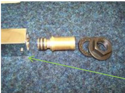
Remove the brass spindle from the spout by loosening grub screw.
