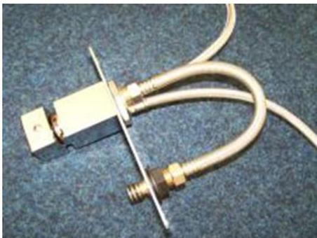
Attach the outlet/spout connection pipe to the connector from the back of the body to the spout thread using the 1/2" BSP flexible pipe. A loop must be made so the pipe can be pushed upwards or downwards into the wall recess.
