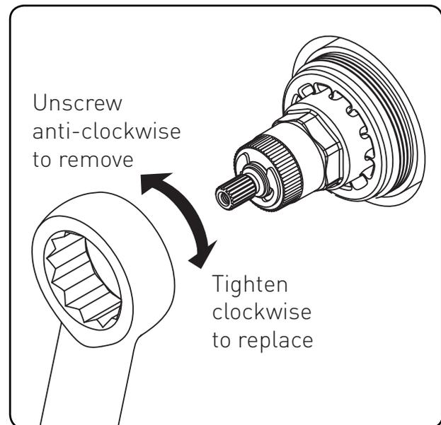
3. Remove the piston and thermostat assembly and place into a bowl. Carefully add hot water (just off the boil) and vinegar to de-scale. Leave in the solution until the water has cooled and rinse with clean water.
