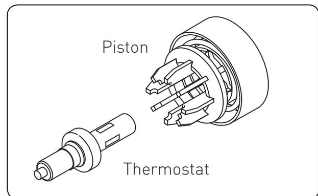
4. Grease the seals with a silicon grease supplied by Bristan (part number: SP-495-0002) and carefully refit.
