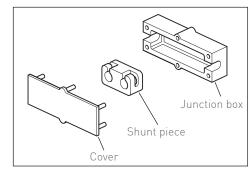
Fit the other end of the extension cable into the extension shunt piece.
