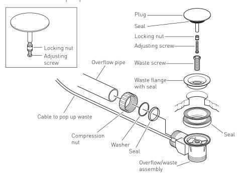
From below push the top part of the rubber seal up through the hole in the bath. Push the waste housing up into the seal and hold in place.
