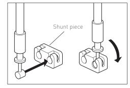
Fit the other end of the original cable in to the extension shunt piece using the same procedure.
