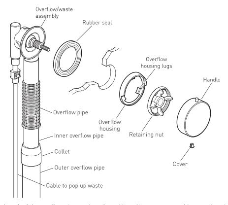
The length of the overflow pipe can be adjusted by pulling apart or pushing together the inner and outer overflow pipes.
