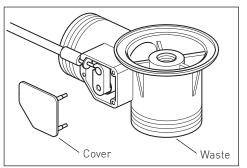
Set the position of the operating lever where the cable connects at 12 o'clock Using a tool for leverage remove the cable collar from the bath waste section and carefully release the cable from the operating lever.
