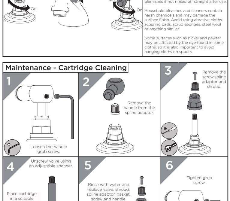
solution and soak until fully de-scaled.
