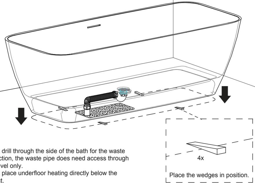
1. Do not drill through the side of the bath for the waste connection, the waste pipe does need access through floor level only.
