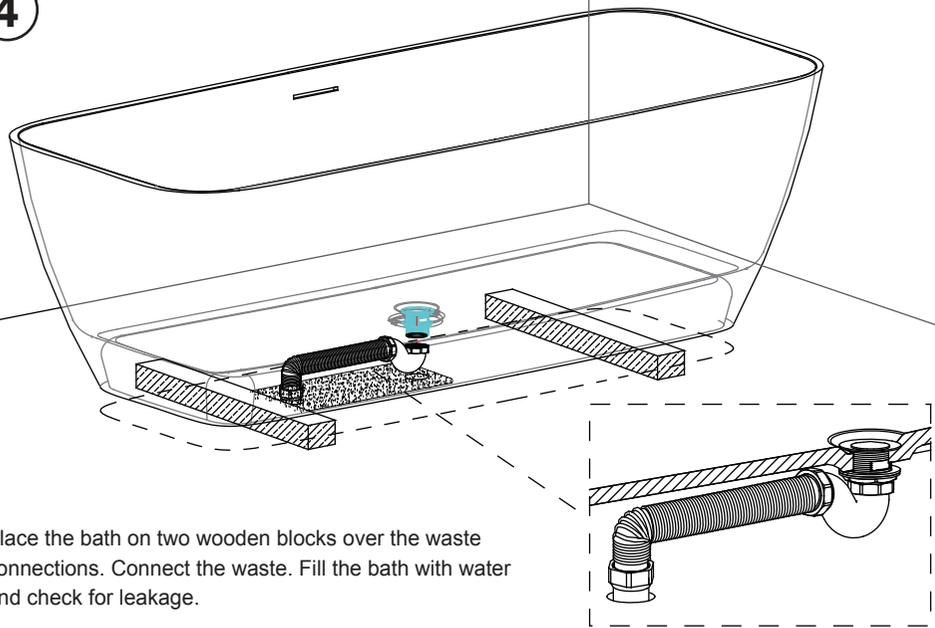
Place the bath on two wooden blocks over the waste connections. Connect the waste. Fill the bath with water and check for leakage.
