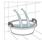
Carefully clean the water pipes before installation
