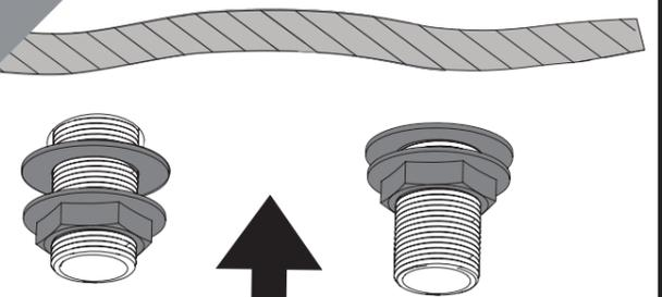
Secure the taps to the basin by using the washer and metal backnut below the basin.
