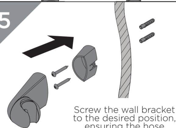
Screw the wall bracket to the desired position, ensuring the hose and handset can reach.
