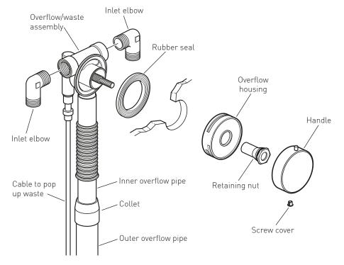
The length of the overflow pipe can be adjusted by pulling apart or pushing together the inner and outer overflow pipes.
