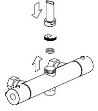
Install the riser into the top outlet of the shower valve.
