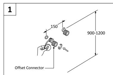
Apply PTFE tape to threads of offset connectors; connect offset connectors onto inlet pipes.
