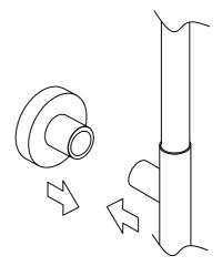
Fit the wall bracket to the riser kit
