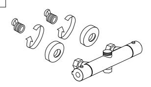
Fit decorative covers over the offset connectors. Then insert sealing washer into nut and tighten onto offset connectors with wrench, being careful not to damage the chrome finish on the connecting nuts.
