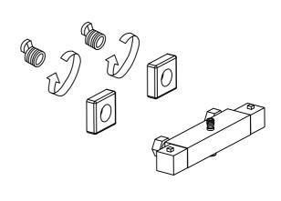
Apply PTFE tape to threads of offset connectors; connect offset connectors onto inlet pipes.
