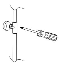
Make sure the riser is level, mark the position of the screw holes on the wall bracket. 6
