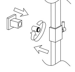
Install the riser into the top outlet of the shower valve.
