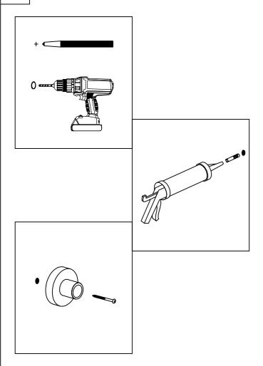
Drill the screw holes and install the wall plugs. To create a seal, apply a small amount of silicone on the inside of the wall plug. 8
