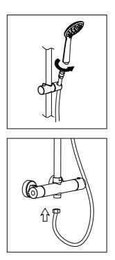
Connect the shower hose to the bottom outlet on the shower valve, and screw the conical end to the shower handset. Place the conical end of the shower flex into the parking bracket on the riser rail.
