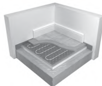
Lay the pipe
