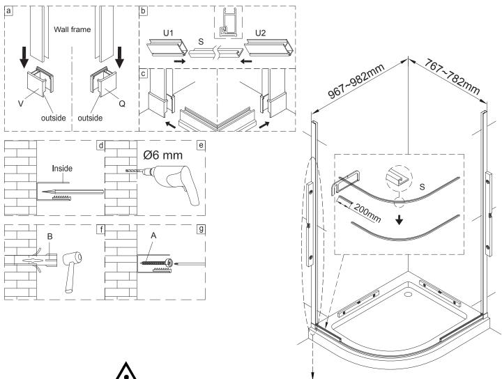
To prevent the moving glass from drooping, the top of wall profile against the moving glass should be 10mm adjusted outward.
