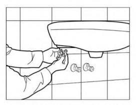
2. The spring fixing washer is installed on washbasin mounting screw and the nut is tightened.
