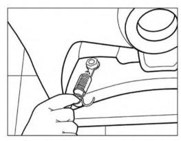
3. The tightening spring end is hooked on the last hole of spring fixing washer and spring stretching ring is held.
