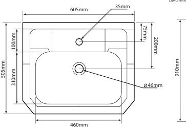
DIAGRAMS NOT TO SCALE | ALL DIMENSIONS IN MM TOLERANCE OF  $\pm$  5MM  ${\rm ALL\ PRODUCTS\ CONFORM\ TO\ BRITISH\ STANDARDS}$
