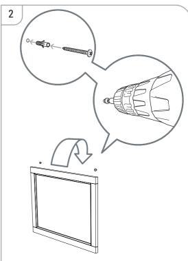
Drill two holes in the marked positions using a 8mm drill bit to a depth of 55mm. Insert the Wall plug supplied and screw in the fixing screw, leaving surfficient head showing to slide into the mirror wall brackets.
