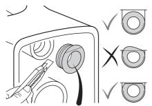
Cut Simpla pan connector to suit if necessary. Apply silicone for better sealing if needed.
