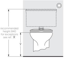
NOTE: For WM closets 840 recommended height from floor to top of cistern is with pan front rim at 400mm. See table for excetions.
