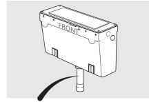
Cut vertical length to suit (cut end with smaller diameter). Allow extra length for elbow and cistern connection.
