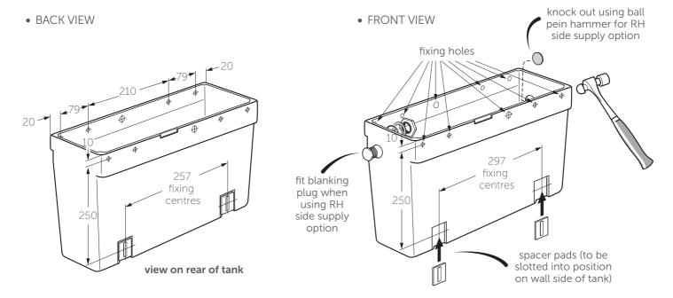
Note: Secure to wall using corrosive resistant fastenings suitable to wall construction (not supplied)
