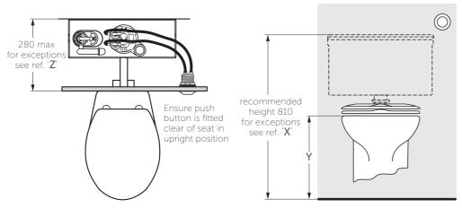
NOTE: For WM closets 810 recommended height from floor to top of cistern is with pan front rim at 400mm. See table for excetions.
