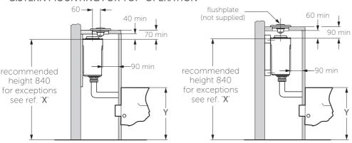
Note: For WM closets 840 recommended height from floor to top of cistern is with pan front rim at 400mm. All dimensions shown in milimetres. Dimensions are approx. and may vary within permitted tolerances.
