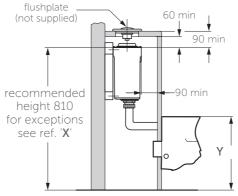
Note: For WM closets 810 recommended height from floor to top of cistern is with pan front rim at 400mm All dimensions shown in milimetres. Dimensions are approx. and may vary within permitted tolerances.
