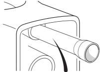
Cut horizontal length to suit (cut end with smaller diameter). Allow extra length for elbow and inlet connector (Simpla).
