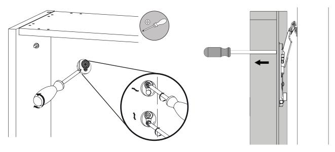
The wall brackets can be adjusted from the inside of the unit.
