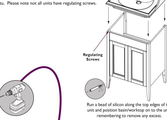
Run a bead of silicon along the top edges of the unit and position basin/worktop on to the unit,
