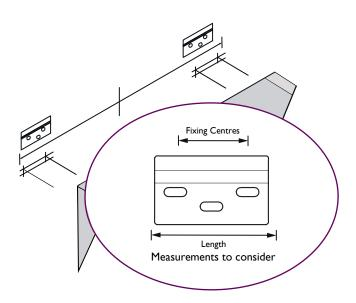
Fit the wall plates to the wall using appropriate fixings (not supplied) using a long spirit level to make sure levelling is accurate. Plates should be no more wide apart than the spanned measurement of the wall hanging brackets.
