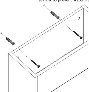
Fasten unit to the wall using suitable bearing screws (not supplied) through the back brace of the unit.
