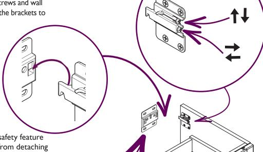
The wall bracket has a safety feature which prevents the unit from detaching from the wall bracket. To unlock this safety feature to remove the unit, press through the hole shown in the image below. This will allow the unit to be removed.
