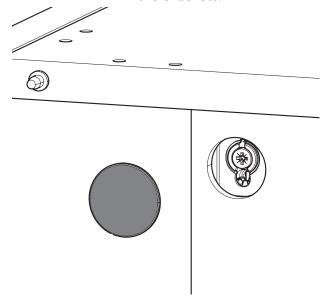
Once adjustments have been completed, the covering caps can be pressed on to conceal all holes.
