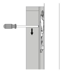
Insert screwdriver into hole below the top screw and turn to move unit up and down, adjust unit for height. By adjusting at both sides the unit can be levelled.
