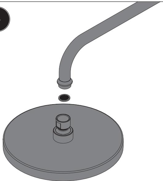
Screw your chosen shower rose onto the shower arm by **HAND ONLY**. Ensure the sealing washer is used.
