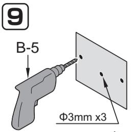
When mounting on a plaster board or tiled wall.
