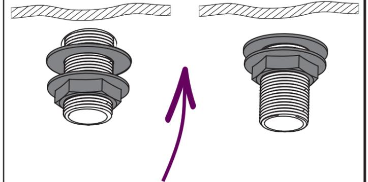
Secure the taps to the bath by using the washer and metal backnut below the bath.
