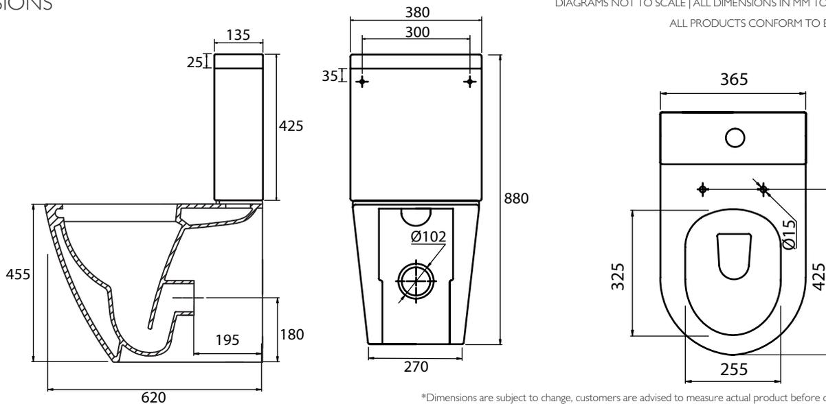
DIAGRAMS NOT TO SCALE | ALL DIMENSIONS IN MM TOLERANCE OF  $\pm 5$ MM
