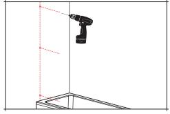
Once the screen is perfectly level in all directions, drill three 3mm holes through the side profile A (Top, centre and bottom of the profile), ensuring to drill through both aluminium profiles but avoiding the glass.
