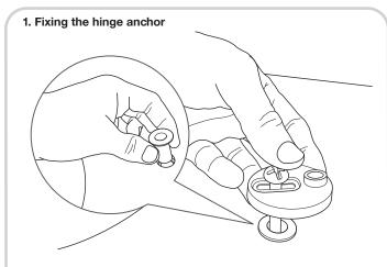
Place the top fix inserts into the fixing holes in the toilet pan. Insert the screws within the hinge anchors as shown and begin to tighten the screws until they are loosely secured, to allow for adjustment of the seat on the pan.
