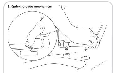
This toilet seat is designed for quick and easy removal when cleaning the toilet pan. To activate the quick release lift the lid and seat up. Press the buttons one by one and lift the seat up. To replace the seat align the sockets with the pins and firmly press down until you hear them click into position.
