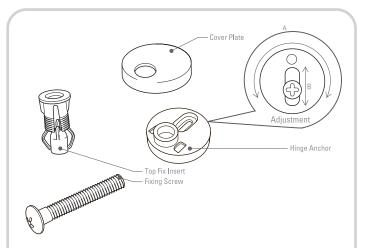
Maximum adjustment of the hinge anchor is achieved by rotating around the screw (adjustment A in the parts diagram above).
