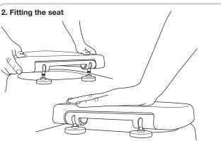
Align and insert the pins into the hinge achors and firmly press down until you hear them 'click' into position.
