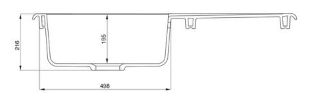
NB: Due to manufacturing processes this sink may have a +/- 3mm tolerance on the measurements.
