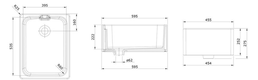
NB: Due to manufacturing processes this sink may have a +/- 5mm tolerance on the measurements.
