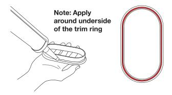
Insert the trim ring into the front side of the fascia. Wipe away any excess silicone around the trim ring.
