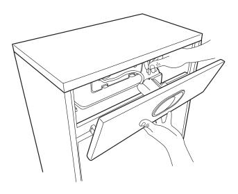
Remove the fascia by unclipping the fascia clips.
