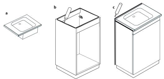
**Note:** Basin waste and taps fittings when over tightened can create stress within the basin material which may in time cause the failure of the product. Waste fittings should be carefully bedded in silicone and the back nut hang tightened an additional quarter turn using a suitable spanner is sufficient to create the required waterlight seal. Care should also be taken when fitting brassware to tap platforms in order to prevent similar stress related failures
