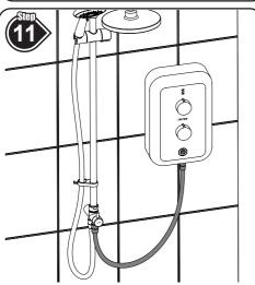
Take the **Short Hose** and fit a hose seal into the conical nut and connect to the **Shower Unit**, fit a hose seal into the conical nut at the other end of the hose and connect to the inlet of the **Diverter Valve**.
