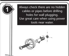
Referring to *Positioning the Dual Outlet Diverter* guidance, mark the wall fixing position for the **Diverter Fixing Bracket** and drill and plug the wall. Ideally the hole should be positioned in the centre of a tile and not in the grouting.
