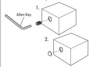
Attach the grub screw to the spindle and secure in position. Place the cover cap on the handles to cover the holes.
