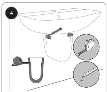
Place your semi-pedestal in position. Trace around the outer edge and mark the position of the fixing holes. Measure the internal width of the ceramic at the back of the pedestal and add the inner line to mark the Pedestal Plumbing Area. Make sure your waste and water connections are in this area.
