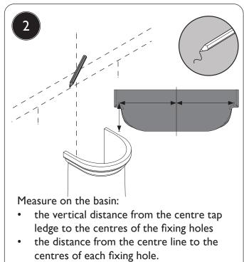
Transfer these measurements on to the wall using the bottom centre of the inverted 'T' as a starting point.
