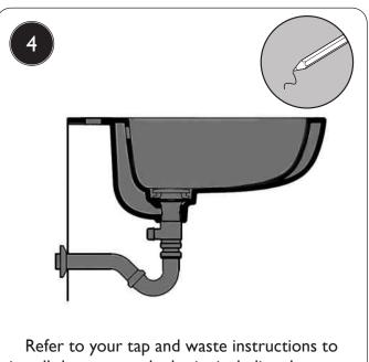
install these on to the basin, including the waste trap. Place the basin back on to the pedestal and mark on the wall the locations of the waste pipework and the hot and cold connections.
