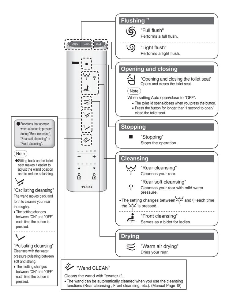
The "Water pressure adjustment", "Wand position adjustment" and "Personal setting" functions are swipe operated.
