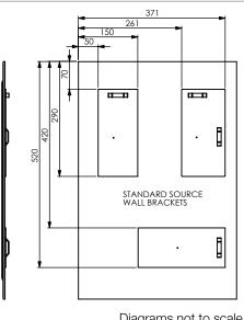
Diagrams not to scale.All dimensions in mm (tolerance of +/-5mm)
