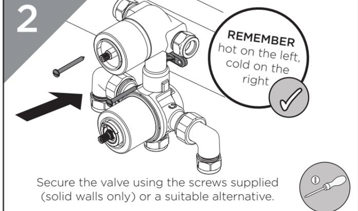
Secure the valve using the screws supplied (solid walls only) or a suitable alternative.
