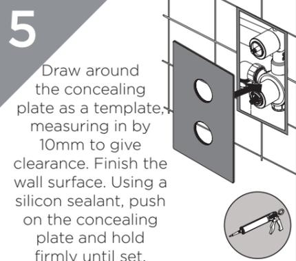
Draw around the concealing plate as a template, measuring in by 10mm to give clearance. Finish the wall surface. Using a silicon sealant, push on the concealing plate and hold firmly until set.
