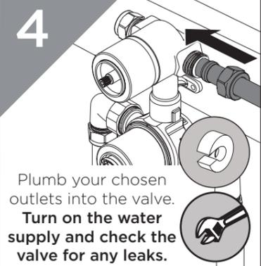
Plumb your chosen outlets into the valve. Turn on the water supply and check the valve for any leaks.
