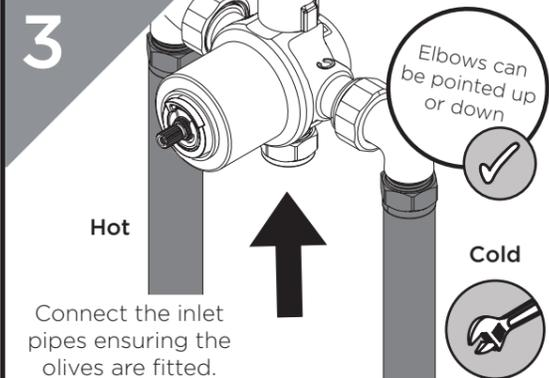
Connect the inlet pipes ensuring the olives are fitted.
