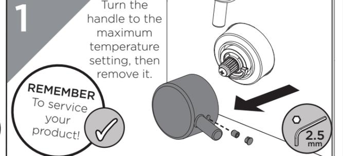
Turn the handle to the maximum temperature setting, then remove it.
