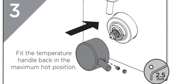
Fit the temperature handle back in the maximum hot position.
