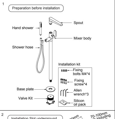
Installation Slot underground size must over 120 x 130 mm, depth 70-100mm including the upper brick
