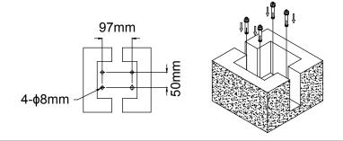
Put in the valve and fasten it with fixing bolts, ensure it is in horizontal measuring by the level.
