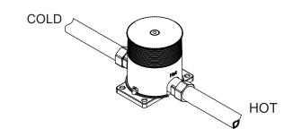
Drilling 4 installation holes at the bottom, then fix and fasten the 4 installation bolts
