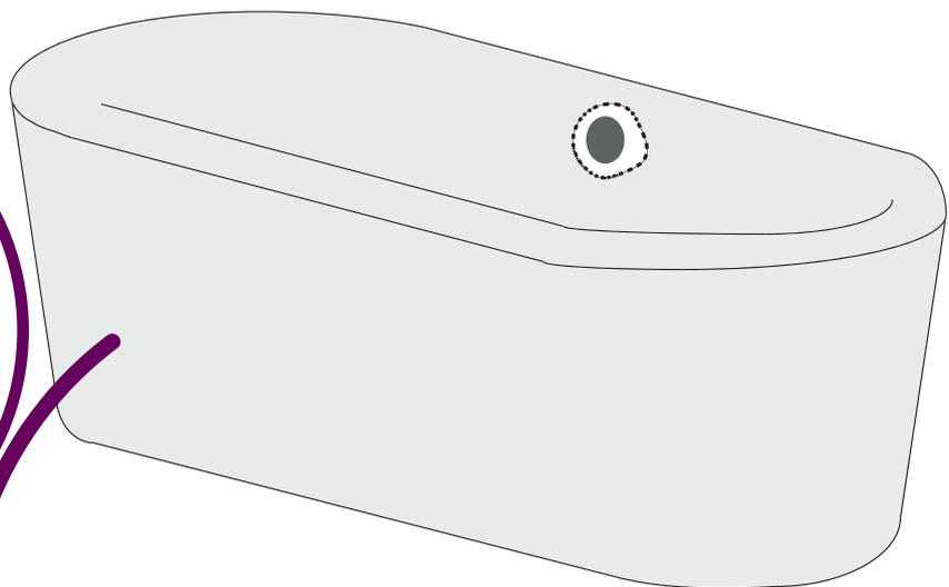
To prepare the bath, carefully place it face up on a dust sheet or protective blanket to prevent damage to the visible areas of the bath. You will also need enough protected space to place the bath on its side or upside down for installation. ⚠ Do not stand in the bath during the installation.
