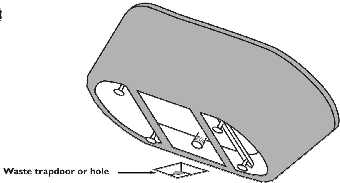
The use of a flexible 40mm waste pipe may be needed once a suitable bath waste trap is fitted.
