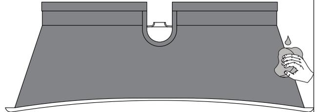
Check the outside surface for any damage and that it is clean and free of any impurities e.g. dirt, dust, grease etc. If cleaning is required, thoroughly clean and degrease the surface with acetone or alcohol. Make sure you allow this to dry before you begin painting.
