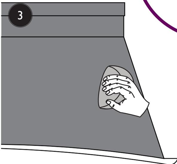
Evenly sand the whole exterior surface using fine sandpaper (320 grain or higher), avoiding where the enamel interior meets the painted surface. This can be done manually or with a sanding machine. Do not excessively sand as this will remove the primer and may cause problems when applying paint.
