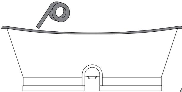
Use masking tape to cover the enamel surfaces at the rim in order to prevent over-spray. Carefully turn the bath tub upside-down on your protected surface.
