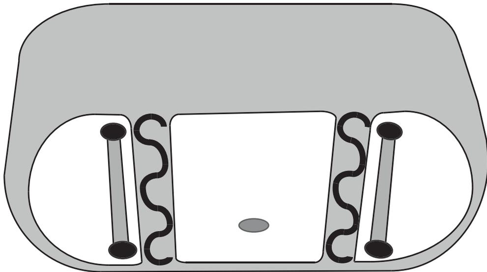
Use a suitable bonding agent (not supplied) and apply to the strengthening bars on the underside of the bath. Equally lower the adjusting feet to the floor; this will stick the bath to the floor.
