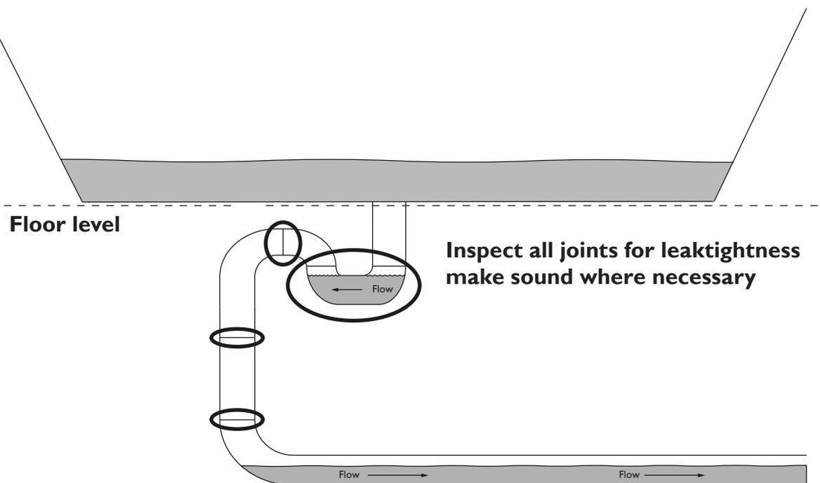
Permanently connect waste and check for leaks by putting some water in the bath and letting it drain.
