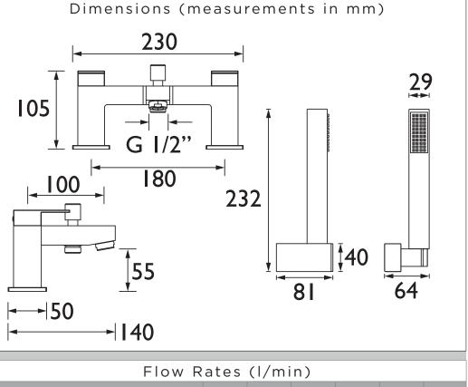
0.5 System Pressure (bar) 0.3 2 3 5 1 18.5 l/min Through Bath Filler (mixed) 20.6 29.2 40.6 57.4 70.3 90.7 Through Handset (mixed) 4.2 5.7 8.7 15.1 18.5 23.8 TECHNICAL DATA
