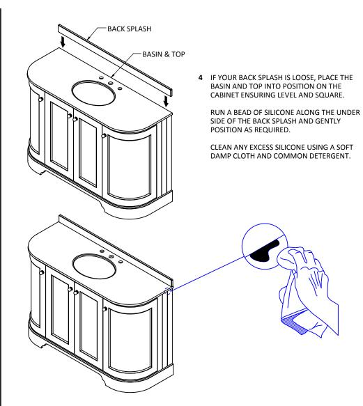
5 ANY EXCESS SILICONE SHOULD BE CLEANED USING A SOFT DAMP CLOTH WITH COMMON DETERGENT.
